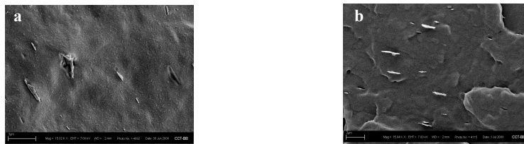
Fig. 2. SEM micrographs at 15000x of a) PP/ 1% A10 and b) PP/ 1% A10T films.
