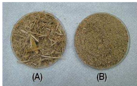
Figure 1. Sugarcane bagasse fibers in nature (A) and modified (B).
