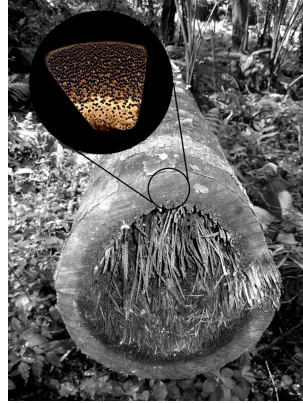
Fig. 6. The stem of the pupunha palm after being cut. The inset highlights the outer region from where a “timber like” material can be obtained. Short fibers can be obtained from inner region.
