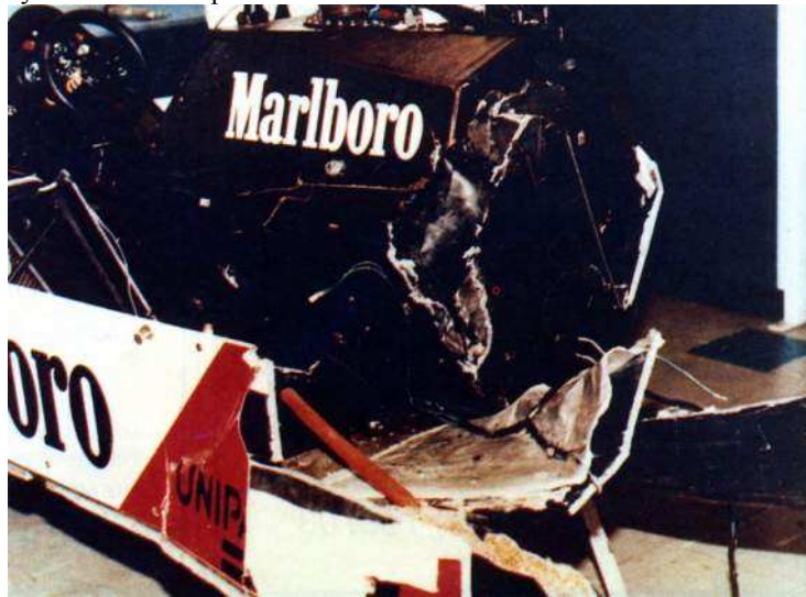
Figure 6: MP4/1 chassis following large impact.
