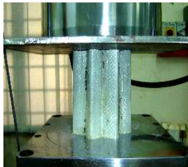
Fig. 1 Tested specimens (composite tubes). Fig. 2 TRCT under compression load
