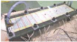
Figure 6. RTM permeability setup.
