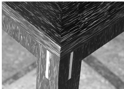
Fig. 7. Visual aspect of the timber like pupunha plank machined along the pupunha trunk length. ( www.lets-evo.net/skateboard/2007/01/23/compensado-de-pupunha ).
