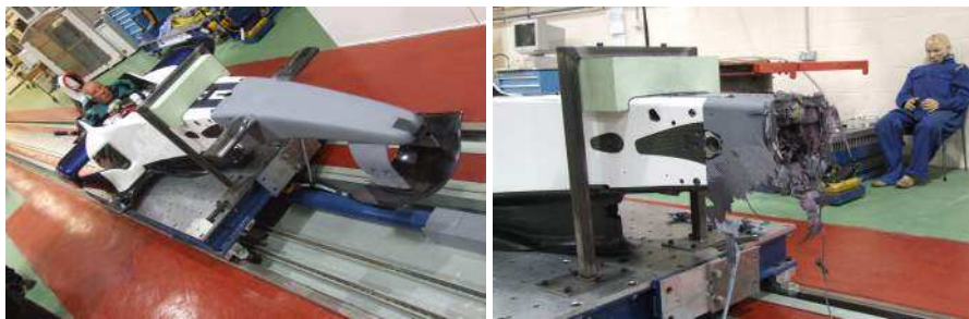
Figure 21: FIA nose crash test.
