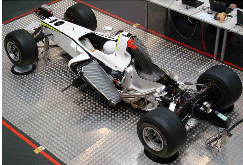
Figure 1 : The “primary structure” of a formula 1 car consists of chassis, engine and gearbox.
