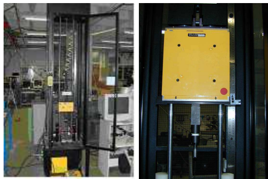
Fig. 1. Drop weight impact test machine. Drop weight and impactor.
