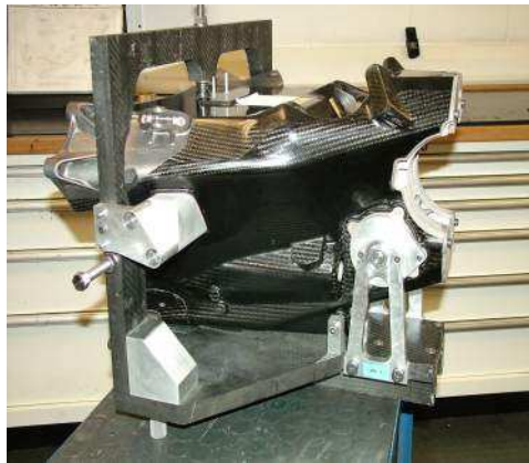
Figure 18: Adhesively bonding a gearbox assembly
