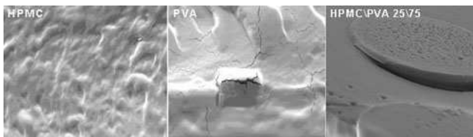
Figure 1. SEM micrographs of polymers HPMC, PVA and HPMC/PVA 25/75 blend (1000x).
