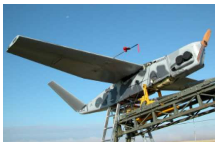
Fig. 1. Left: UAV SIVA in a pneumatic launch ramp. Right: sketch of the installed monitoring system.
