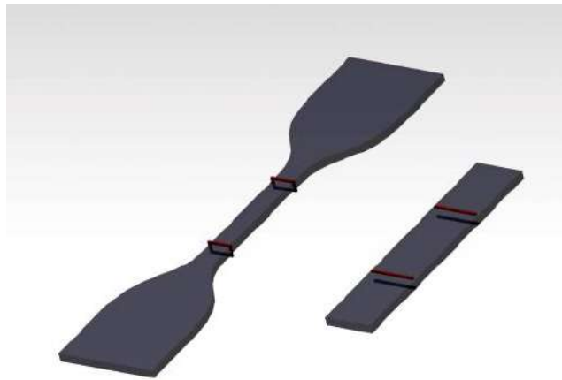
Figure 2.4: Schematics of electrode disposition in tensile (left) and flexure (right) coupons.
