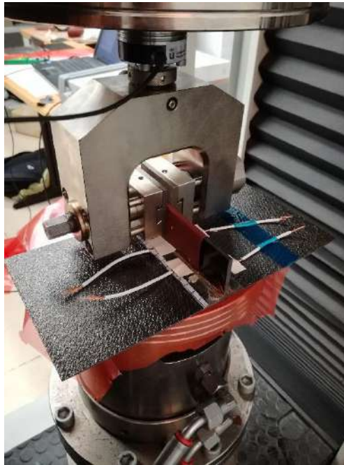
Figure 2.13: Image of the actual configuration for skin-stringer peeling tests.
